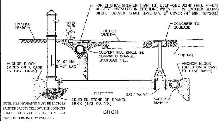
NOTE: ALL FIRE HYDRANTS SHALL HAVE THRUST BLOCKS AND JOINT RESTRAINTS FROM HYDRANT TO WATERMAIN.
