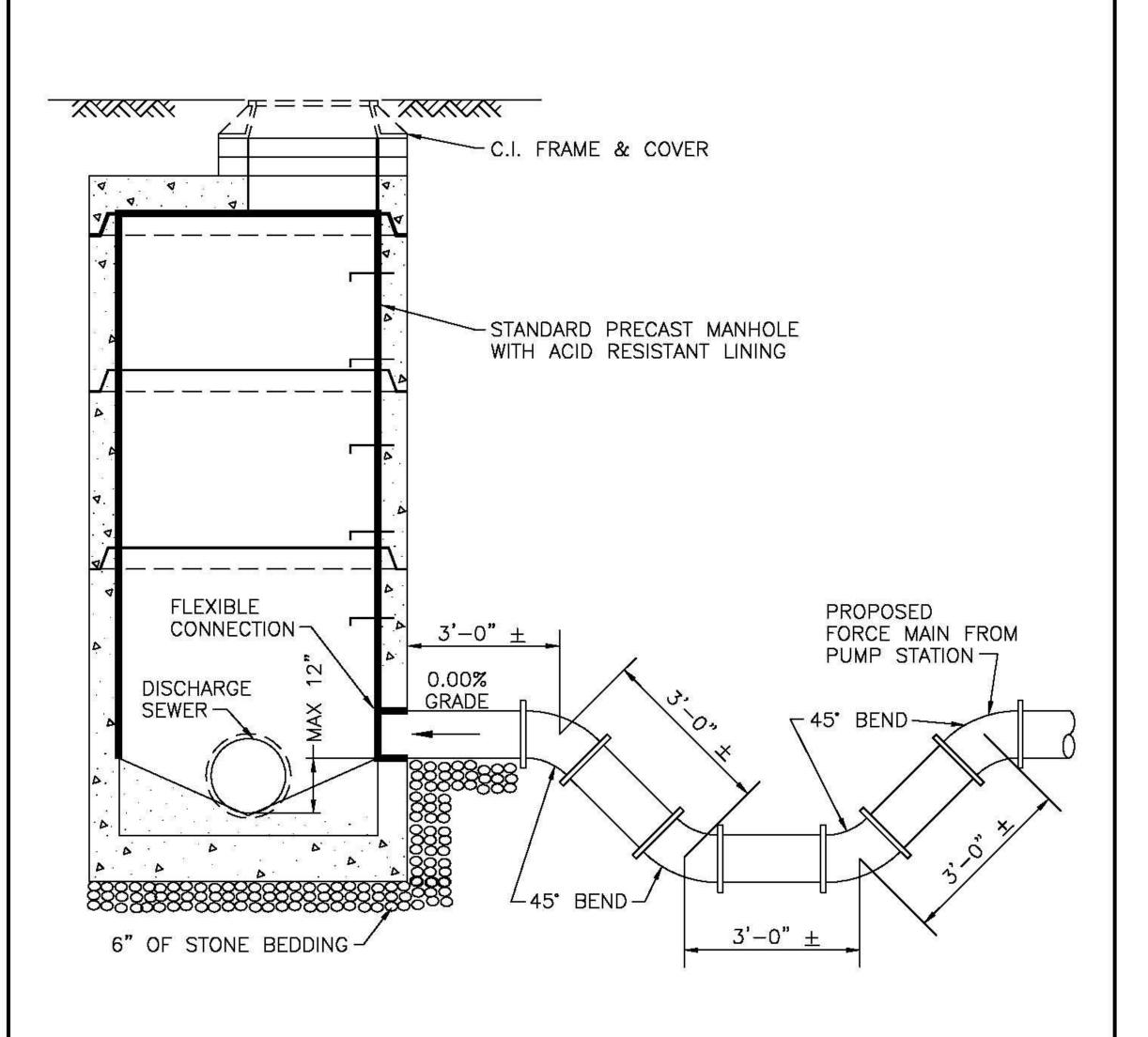
NOTE: USE SULFATE RESISTANT CEMENT TO PREPARE MOTAR IN BUILDING INVERT & BENCH.
